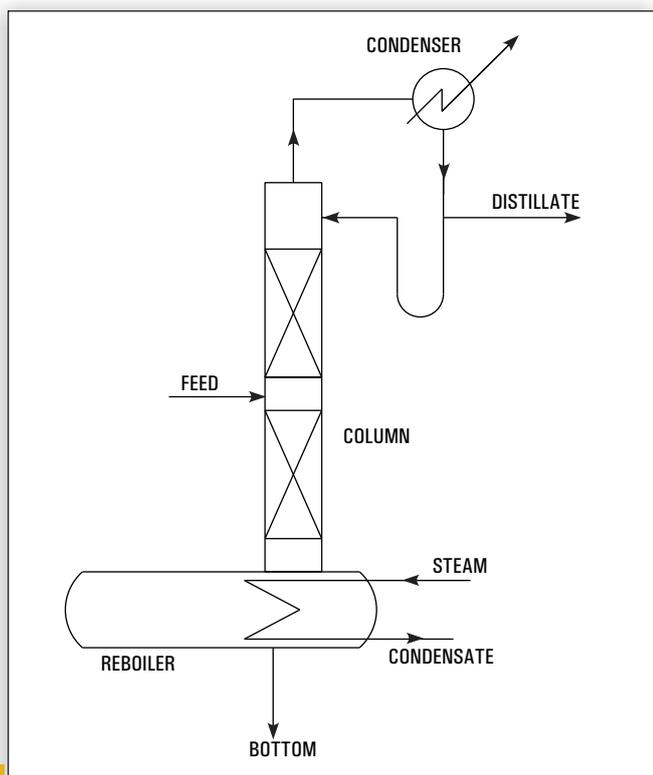
The limitations of batch distillations are naturally circumvented in continuous distillation as shown in fig.2 which is a typical fractionating unit comprising of ratification & stripping sections. Here feed is continuously fed to the column with withdrawal of top & bottom products. The process takes care on its own by simply maintaining the flow rates of feed & utilities.
